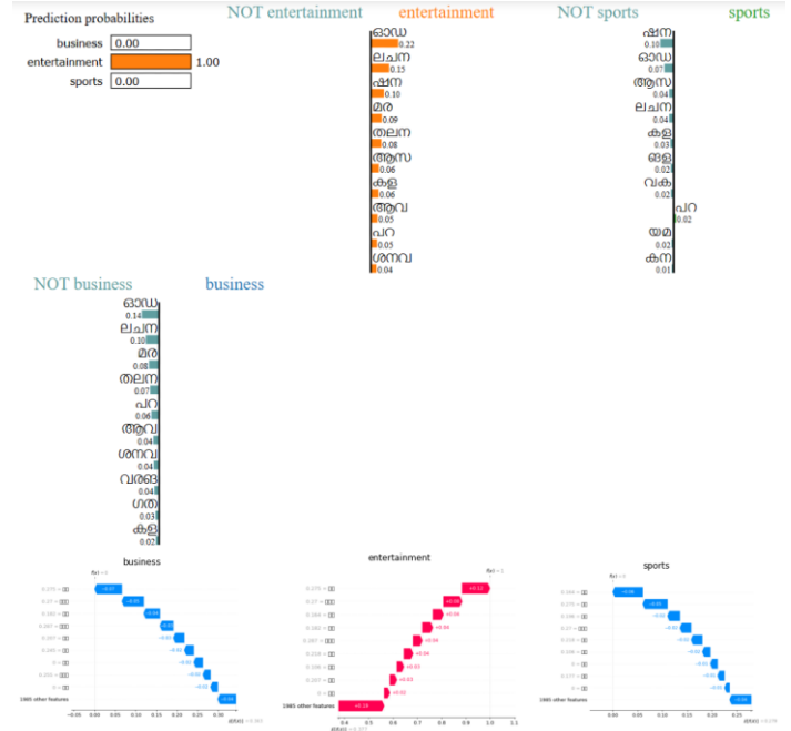
Fig.7. LIME plot and SHAP waterfall plot explaining the choice of the class for a sample data item in Malayalam news headline dataset
