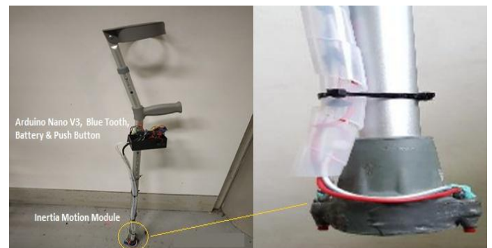
Fig.3. Mechanical Cane Design with Inertia Motion Sensor
