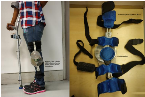
Fig.4. Cane Controlled Knee Exoskeleton Robot
