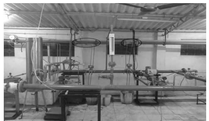
Fig.A1. Experimental setup with leak position 1 & 2 near flow nozzle and Venturi (encircled)
