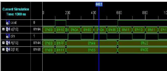
Fig.6. Output of 8-bit CLA Adder
