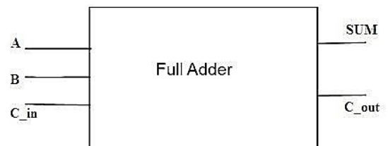
Fig.1. Basic building block of 1-bit full Adder cell
