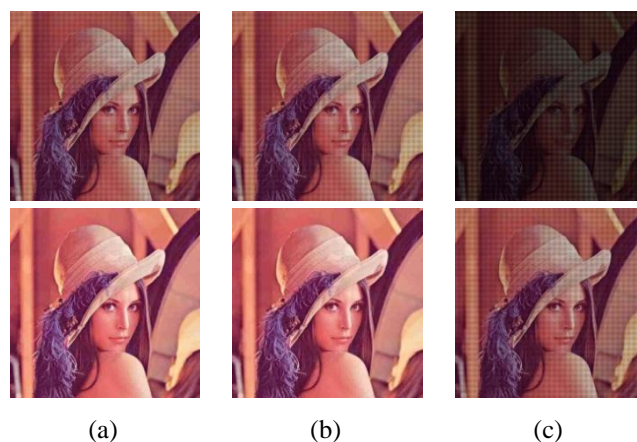
Fig. 1. (a) Odd and Even-Numbered Rows (b) Odd and Even-Numbered Columns (c) Odd and Even-Numbered Rows and Columns
