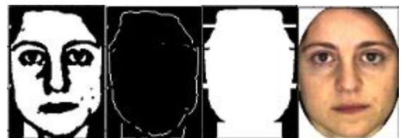
Fig.4. a) CLAHE plus Global Otsu b) Outer border c) Filled area d) Elliptical face image.
