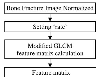
Fig.2. Calculation process of Modified-GLCM algorithm
