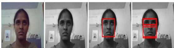
Fig.6. Detection of mouth in closed position
