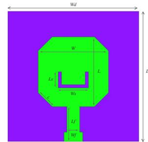
Fig.1.(a) Front view of octagonal antenna with U-shaped slot and Microstrip Feed
