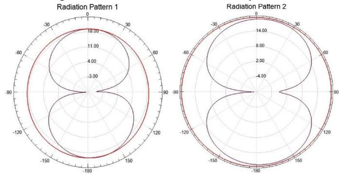
Fig.5. Radiation Pattern at (a) E Plane and (b) H Plane
