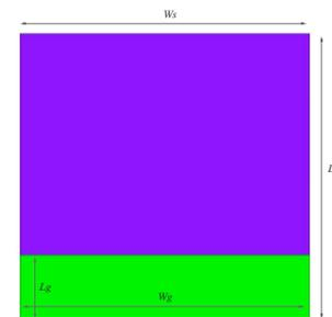
Fig.1.(b) Back view of patch antenna with Defective Ground Structure (DGS)
