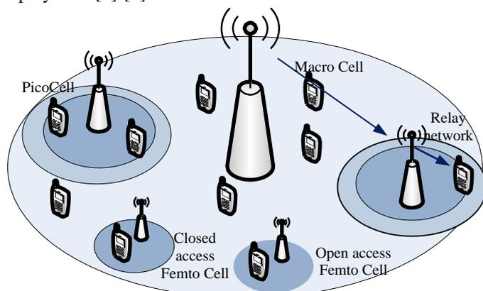
Fig.1. Heterogeneous network with both high-power (macro-cell base station) and low-power (pico-cell base station, etc.) nodes
