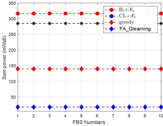
Fig.5. Performance comparison of sum transmit power of the FBSs for different methods
