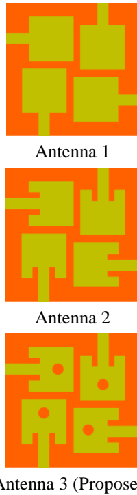
Fig.1 Step-wise evolution of the Antenna-1, Antenna-2 and Antenna-3 (Proposed)
