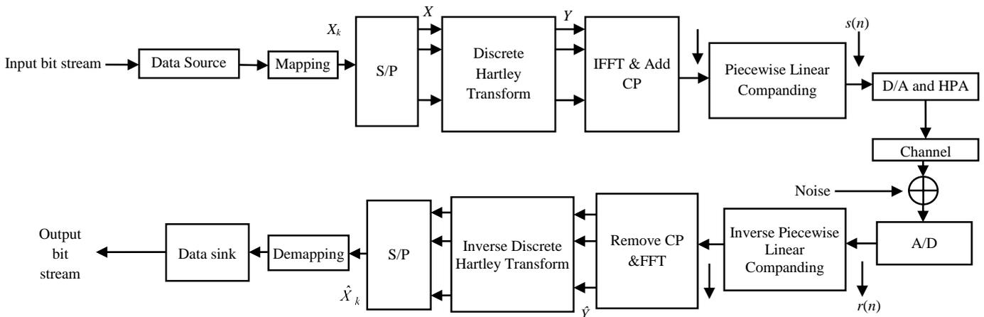
Fig.2. Block diagram of OFDM system with DHT and Piecewise Companding
