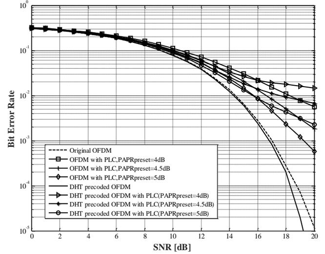
Fig.8. BER Performance of original OFDM signal and different techniques with SSPA over AWGN channel with 16-QAM modulation
