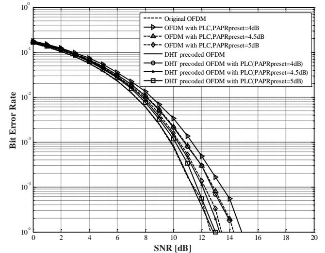
Fig.5. BER Performance of original OFDM signal and different techniques over AWGN channel with 4-QAM modulation
