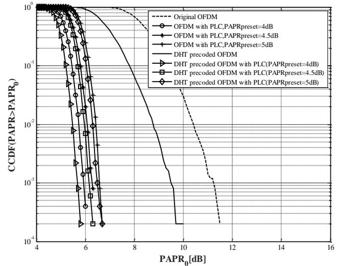
Fig.4. CCDFs of original OFDM signal and different PAPR reduction techniques with 16-QAM modulation
