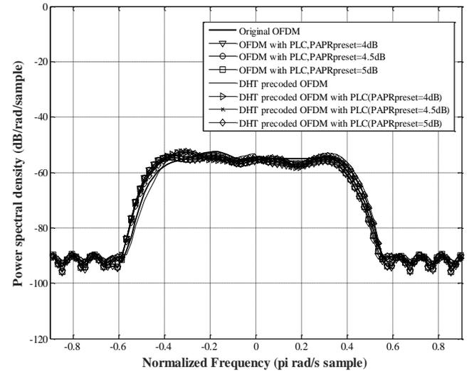
Fig.9. PSD's of original OFDM signal and different PAPR reduction techniques with 4-QAM modulation
