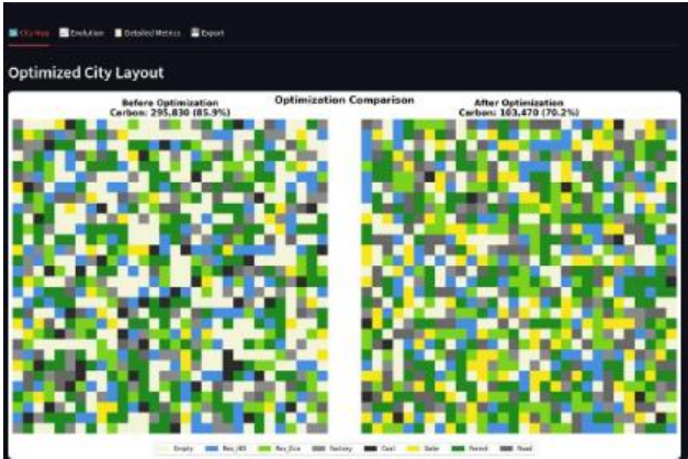
Fig.1. Before (initial random layout) and after (optimized layout at convergence) for a representative 50×50 run. The optimized city shows increased forest coverage, solar farm clusters, and improved residential-to-green-space proximity
