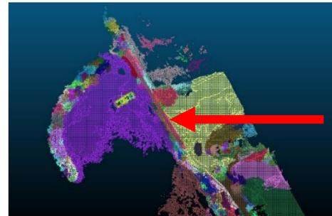
Fig.11. Pink strip down middle of breakwater defines crest as shown by red arrow. Segmentation done with distance threshold parameter set to 5, colorimetric difference between points set to 8, region merging threshold set to 5. Higher values for these parameters equate to a higher allowable colorimetric distance for both points and regions, and therefore a lower level of segmentation and vice versa.
