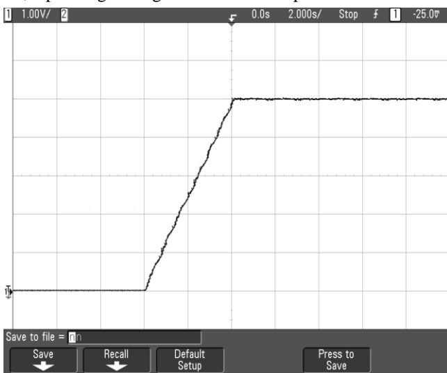
Fig.12. Experimental output of step change in reference speed from zero to rated speed
