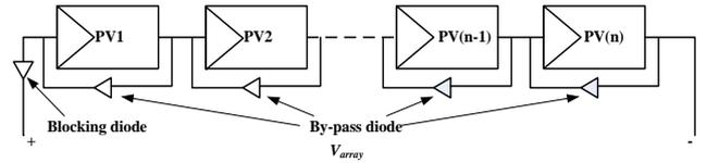
Fig.2. PV Array Formed by  $n$  Series Connected PV Modules
