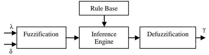
Fig.4. Basic Elements in Fuzzy Logic Control
