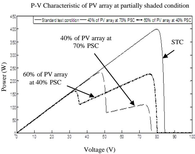
Fig.8. P-V Characteristics of PV Arrays under PSC
