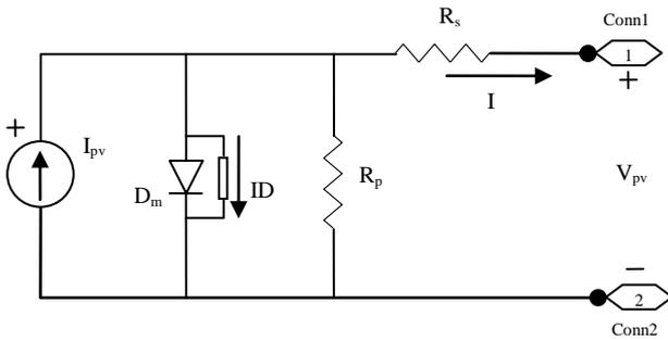
Fig.1. One Diode Model
