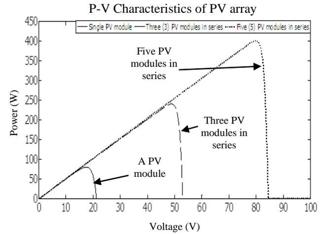
Fig.6. P-V Characteristics of PV Arrays under STC
