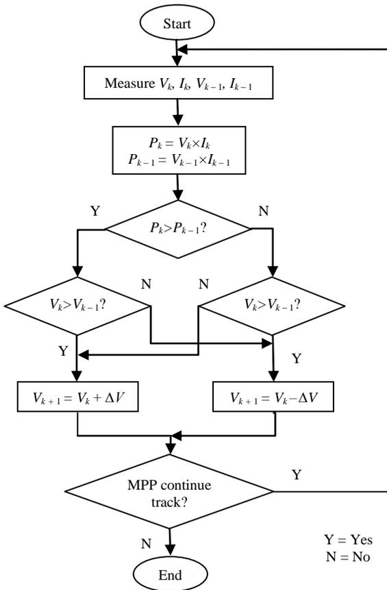
Fig.3. Flowchart of P&O Control Algorithm
