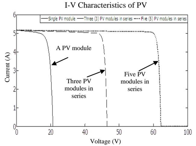
Fig.5. I-V Characteristics of PV Arrays under STC
