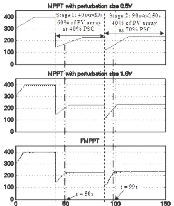
Fig.9. The Output Power Controlled by MPPT and FMPPT
