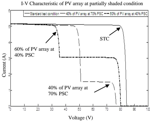
Fig.7. I-V Characteristics of PV Arrays under PSC
