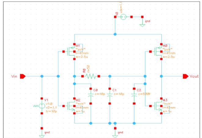
Fig.9. Schematic of two CMOS gate interconnect circuit
