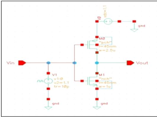
Fig.3. Implemented schematic of an inverter in cadence software using 45nm technology
