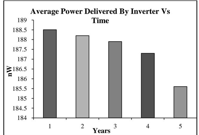
Fig.8. Reliability analysis of inverter in terms of average power delivered and time
