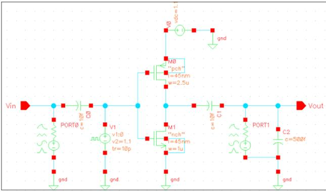
Fig.6. Schematic of inverter for noise analysis using ports at both terminals at 5GHz frequency
