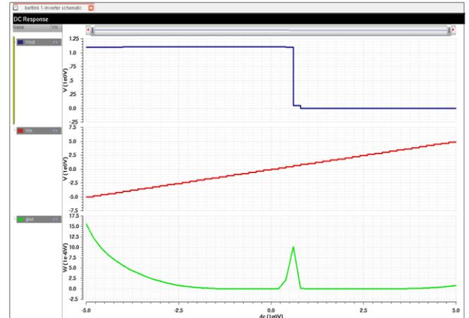
Fig.5. DC response of inverter ( $V_{\text{out}}$ ,  $V_{\text{in}}$  & Power of the Inverter)
