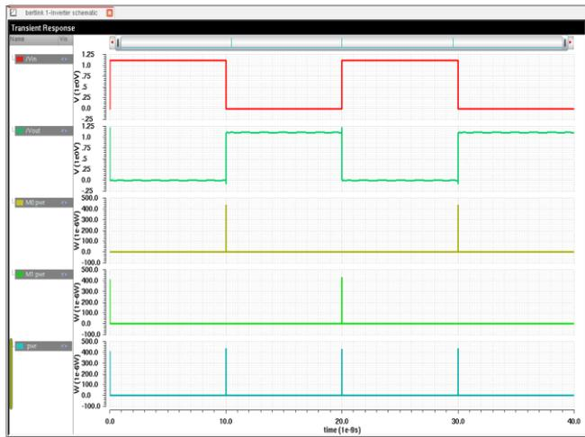
Fig.4. Transient response of an inverter ( $V_{\text{in}}$ ,  $V_{\text{out}}$ , Power of PMOS, Power of NMOS & Power of the Inverter)
