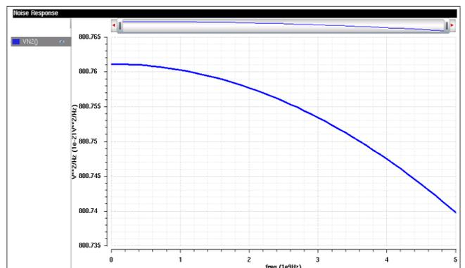
Fig.13. Noise response of two CMOS gate @ 5GHz
