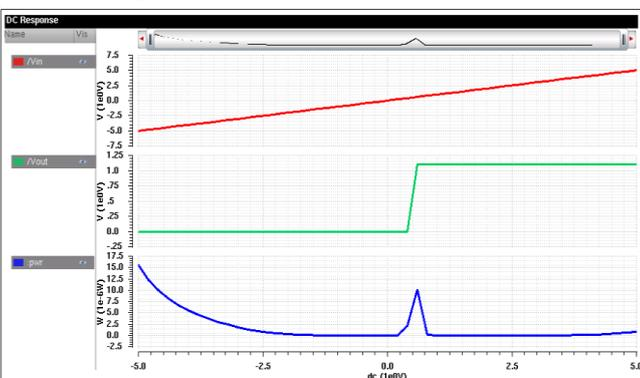
Fig.11. DC response of two CMOS gate interconnect circuit ( $V_{in}$ ,  $V_{out}$  & Power of the circuit)
