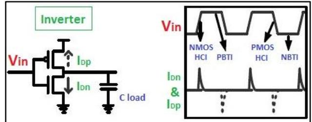
Fig.2. Schematic of an inverter circuit
