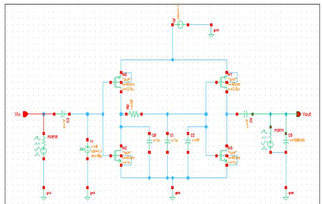
Fig.12. Schematic of two CMOS gate for noise analysis using ports at both terminals @ 5GHz
