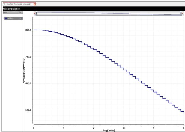
Fig.7. Noise response of inverter at operational frequency of 5GHz
