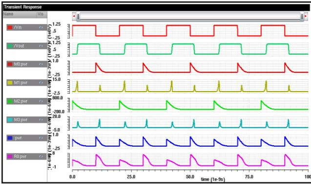
Fig.10. Transient response of two CMOS gate interconnect circuit ( $V_{in}$ ,  $V_{out}$ , power consumed by Mo, M1, M2, M3, Power of the circuit & power consumed by of resistance)
