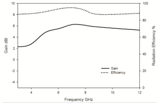
Fig.11. Measured efficiency and Gain
