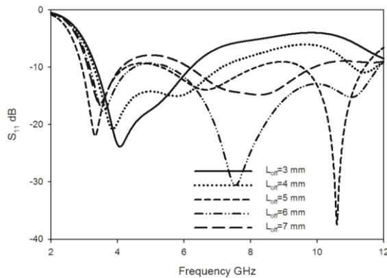
Fig.4. Effect of  $L_{off}$  on  $S_{11}$
