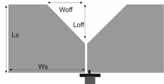
Fig 1. Proposed Antenna Structure
