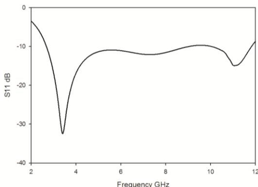
Fig.15. Reflection coefficient obtained using FDTD
