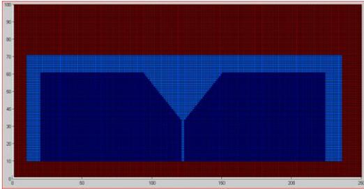
Fig.14 Computation field of Proposed UWB antenna in FDTD
