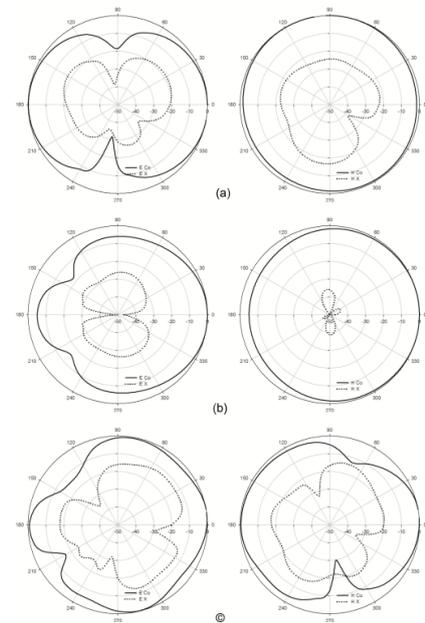
Fig.8. E and H plane Radiation patterns at three resonances
