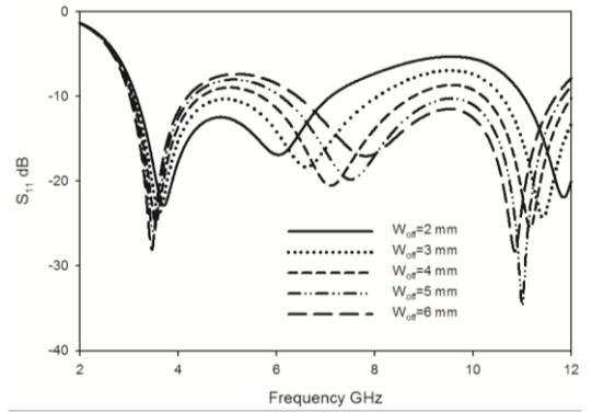
Fig.5. Effect of  $W_{off}$  on  $S_{11}$
