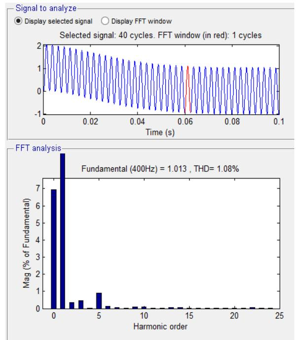
Fig.9. Harmonic Spectrum of Source Current of aircraft system with SAPF
