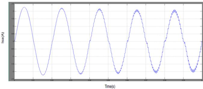
Fig.6. Source current for nonlinear load before compensation
