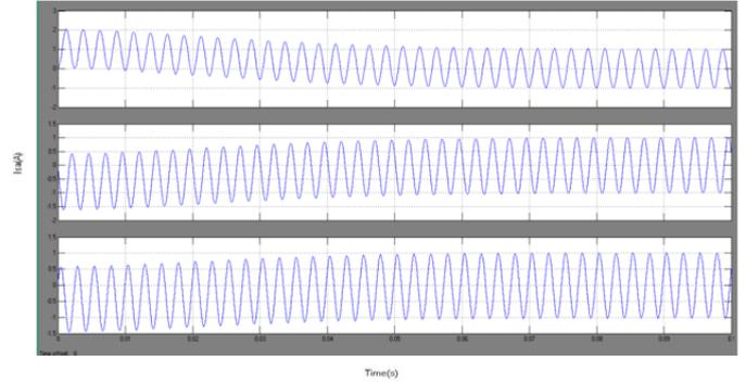
Fig.7. Source current for nonlinear load after compensation
