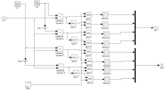
Fig.4. Gating Signal Generation by CPS-PWM
