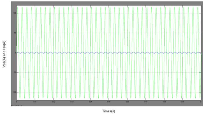
Fig.8. Source voltage and current of aircraft system after compensation
