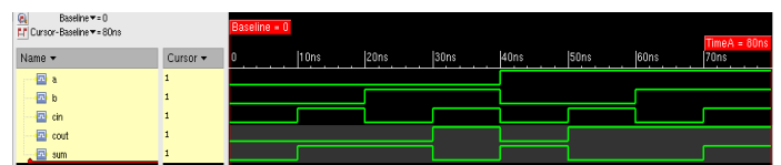
Fig.10. Simulated waveform of proposed RCSFAs
