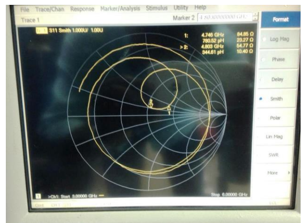
Fig.11. Smith chart of Dual Element Microstrip Antenna showing resonating impedance 54.77Ω
