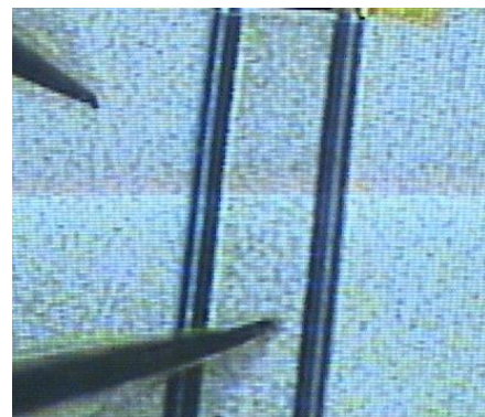
Fig.4. RF probing of CPW line
