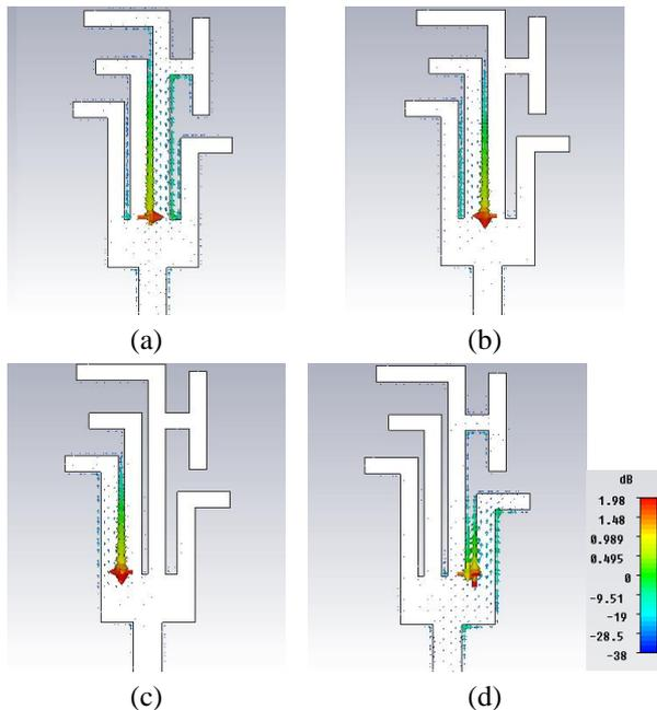
Fig.6. Surface current distributions at frequency (a) 2.54GHz (b) 3.51GHz (c) 4.38GHz (d) 5.3GHz
