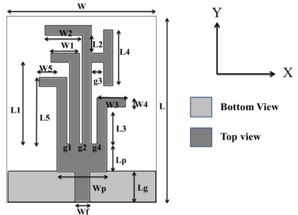
Fig.1. Geometry of proposed compact printed Quad band antenna
