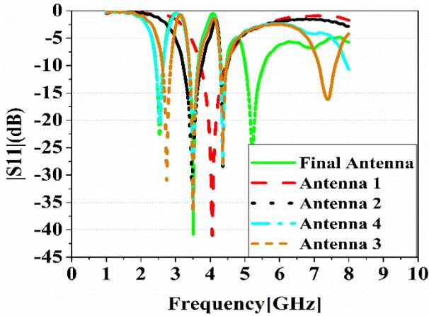
Fig.5 |S<sub>11</sub>| against frequency for above all antenna
