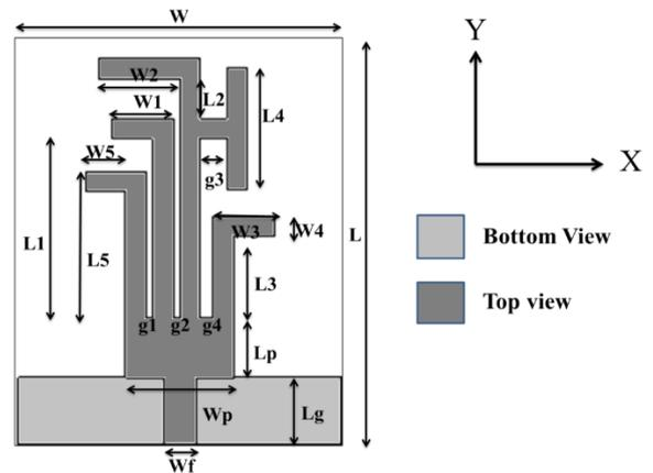
Fig.1. Geometry of proposed compact printed Quad band antenna
