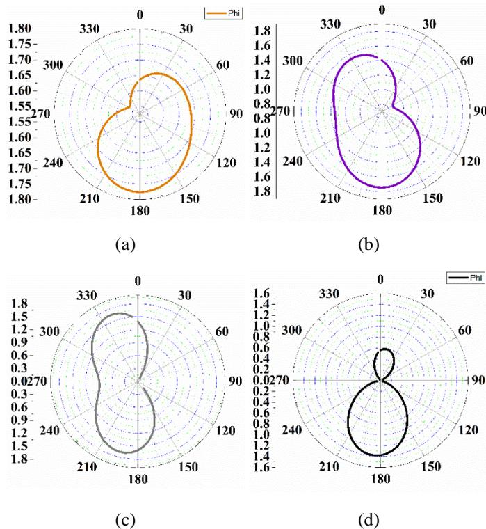
Fig.12. Radiation pattern of proposed antenna at resonance frequencies (a) 2.54GHz (b) 3.51GHz (c) 4.38GHz (d) 5.3GHz
