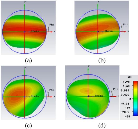
Fig.11. 3D-Radiation pattern of proposed antenna at resonance frequencies (a) 2.54GHz (b) 3.51GHz (c) 4.38GHz (d) 5.3GHz
