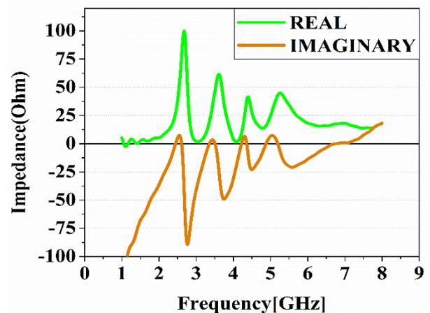
Fig.4. Input impedance against frequency
