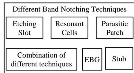
Fig.1. Band notching techniques
