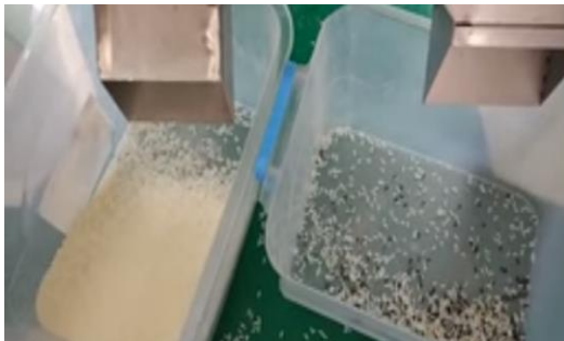
Fig.21. Separating defective and non-defective rice
