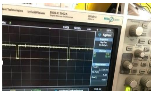
Fig.16. Clock Generation of the Grain Sorting Machine
