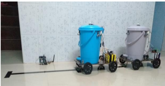
Fig.4. Proposed Self-Monitoring Automated Route Trash (SMART) Dustbin
