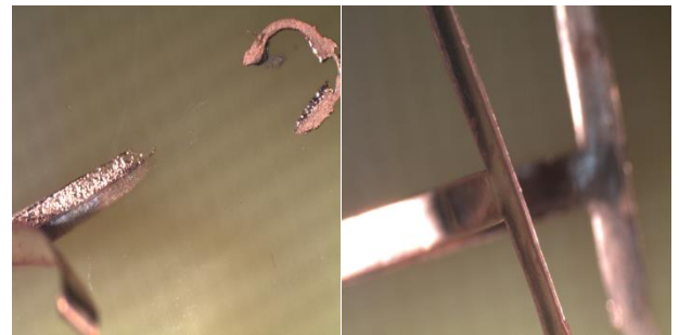
Fig.6. Optical photographs of peeled electroplated copper from base copper, in which freshly prepared ammonium persulphate acts as micro-etchant
