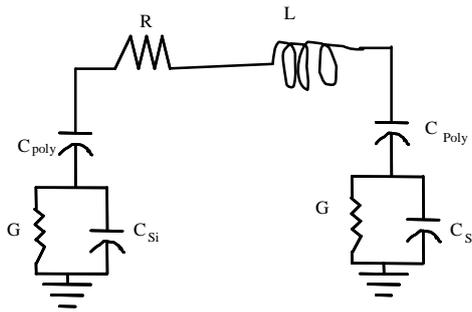
Fig.1. Transmission line equivalence
