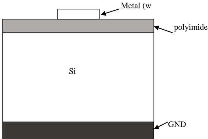
Fig.4. Cross section schematic of transmission line
