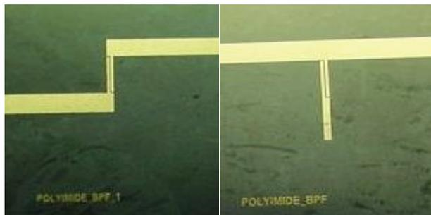
Fig.6. Fabricated BPF topology over polyimide
