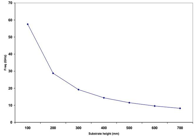
Fig.3. Effect of substrate thickness on the cut off frequency
