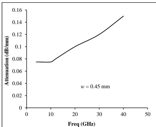
Fig.5. Simulation study of the attenuation characteristics of polyimide based TL
