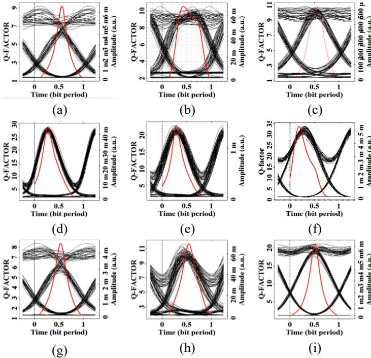
Fig.6. Eye-diagrams for: (a), (b), (c) pre, post, symmetric-compensation with NRZ; (d), (e), (f) pre, post, symmetric-compensation with RZ; (g), (h), (i) pre, post and symmetric-compensation with Gaussian lone codes, respectively
