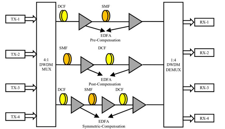
Fig.4. Principal of 4-channels DWDM optical transmission system
