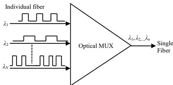
Fig.1. Basic building block of optical DWDM transmission system
