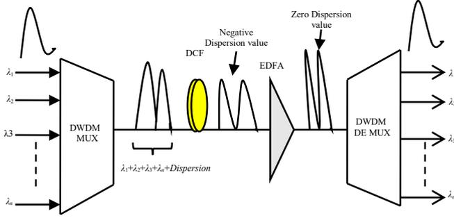
Fig.3. Basic principal of DCF Technique with EDFA-DWDM optical transmission system
