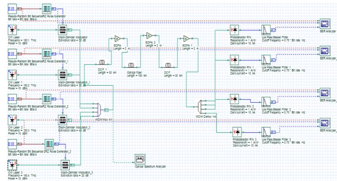
Fig.5. Proposed simulation model of 4×8 GBPS DWDM optical transmission system
