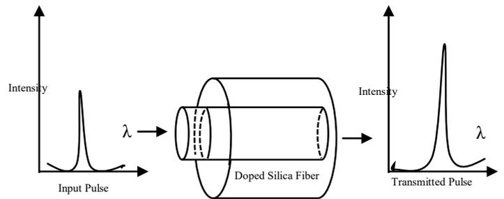
Fig.2. Basic principal of EDFA amplifier
