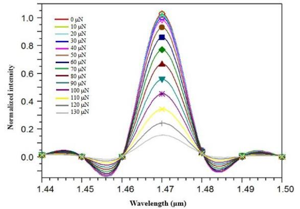
Fig.8. Normalized Transmission Spectrum of the Proposed Sensor of Force (0-130 $\mu\text{N}$ )
