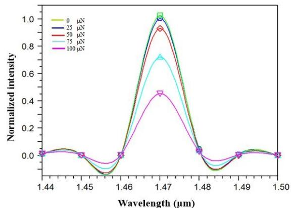
Fig.9. Normalized Transmission Spectrum of the Proposed Sensor of Force (0-100 $\mu\text{N}$ )
