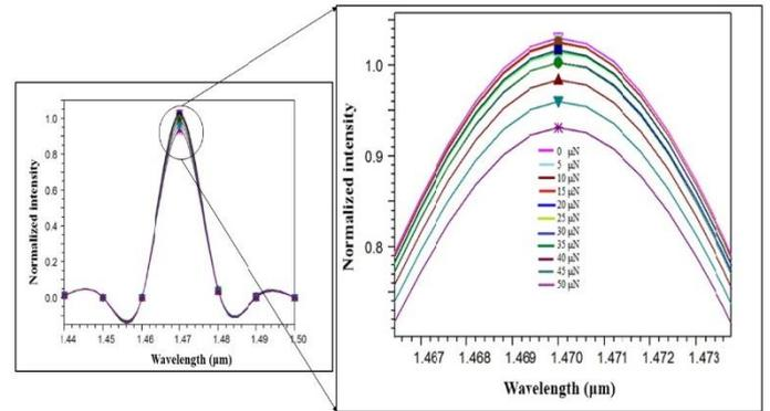
Fig.7. Normalized Transmission Spectrum of the Proposed Sensor of Force (0-50 $\mu\text{N}$ )
