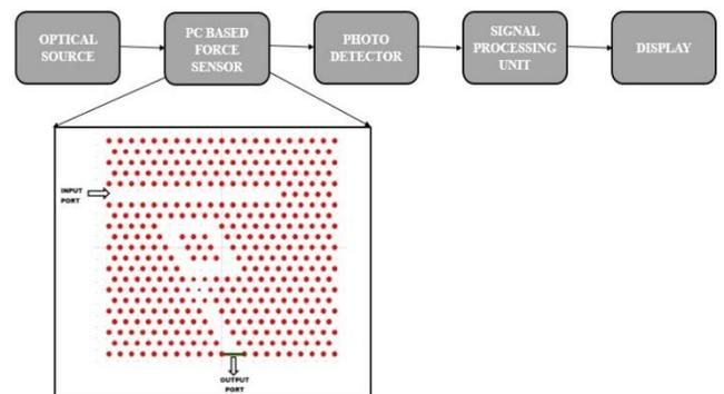
Fig.4. Schematic Structure of Force Sensor
