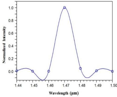
Fig.5. Normalized Transmission Spectrum of the Proposed Sensor
