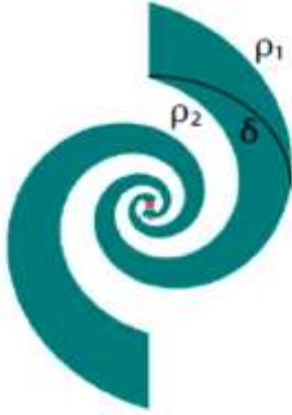
Fig.3. Equiangular spiral antenna [17]
