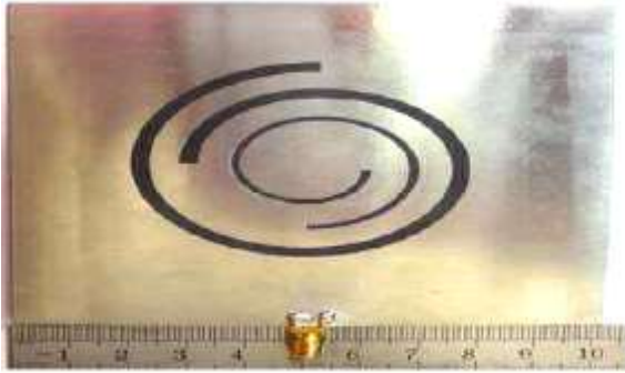
Fig.5. Spiral Antenna Design for CNSS [18]
