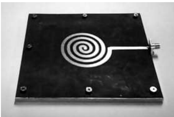
Fig.9. A single arm spiral antenna with Micro-strip Line Feed [24]
