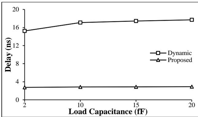
Fig.7. Delay of the Comparators with Load Capacitance
