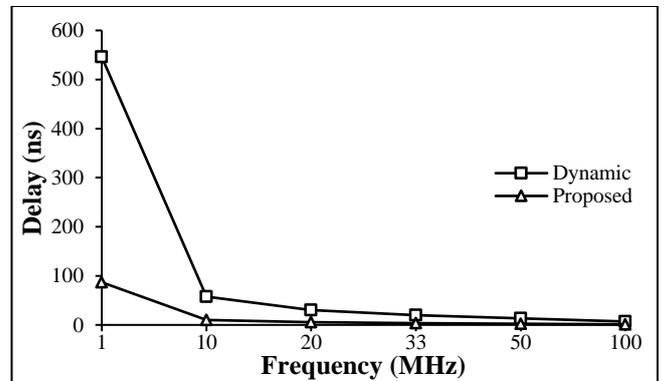
Fig.5. Delay of the Comparators with frequency
