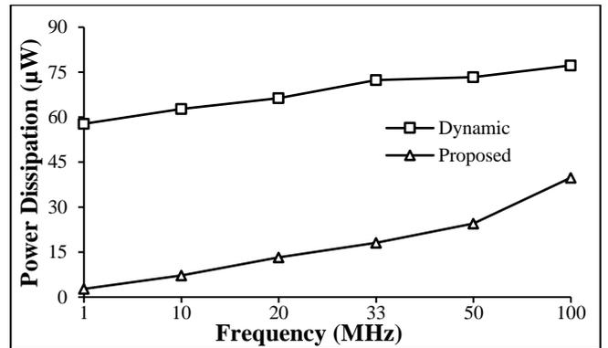
Fig.4. Power Dissipation of the Comparators with frequency
