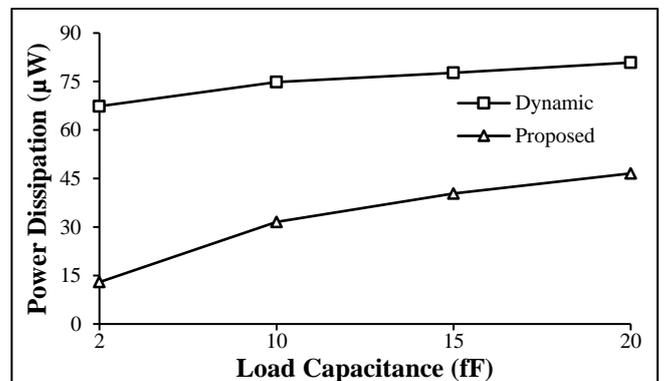
Fig.6. Power Dissipation of the Comparators with Load Capacitance
