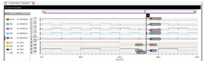
Fig.4. Simulation waveforms of 1-Digit BCD Adder
