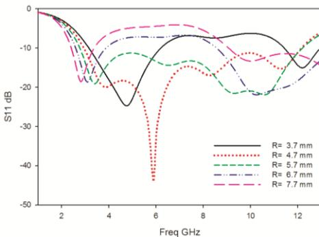
Fig.4. Effect of R on Resonant frequency
