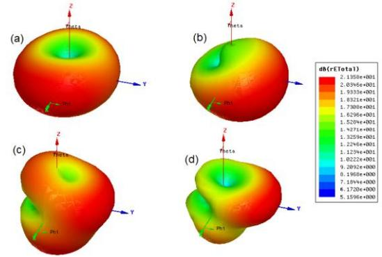
Fig.8. Simulated Radiation pattern at resonances
