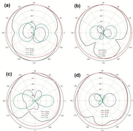
Fig.7. Measured Radiation pattern at resonances
