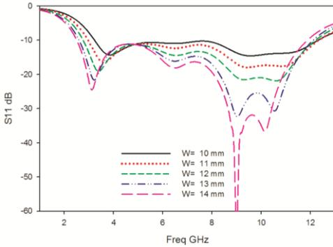
Fig.3. Effect of W on Resonant frequency
