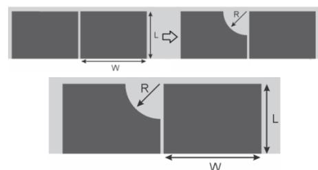
Fig.1. Evolution and Derived Structure of UWB Antenna
