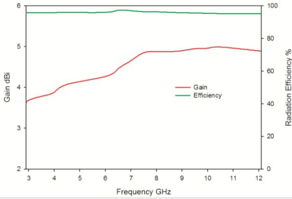
Fig.10. Measured Efficiency and Gain
