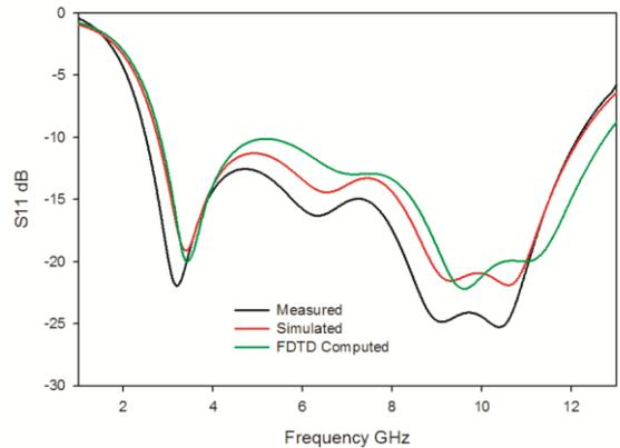
Fig.13. Comparison of Measured and FDTD calculated S11
