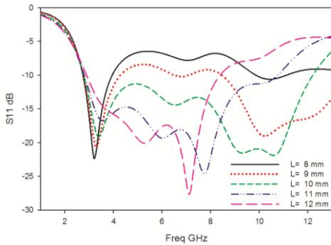
Fig.2. Effect of L on Resonant frequency
