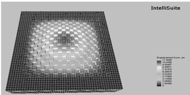
Fig.18. Simulation of perforated Si-diaphragm deformation on the Z axis with maximum pressure of 0.3MPa
