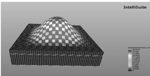
Fig.20. Mises Stress analysis of the perforated Si-diaphragm with Pressure of 0.7Mpa
