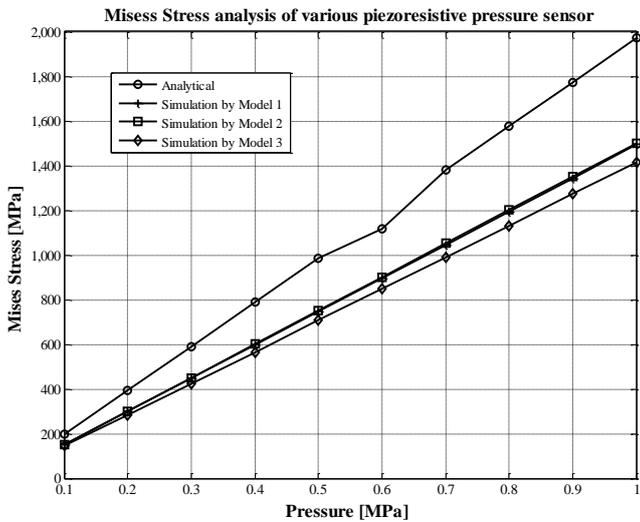
Fig.14. Mises stress analysis of various piezoresistive pressure sensors with thickness at 5µm
