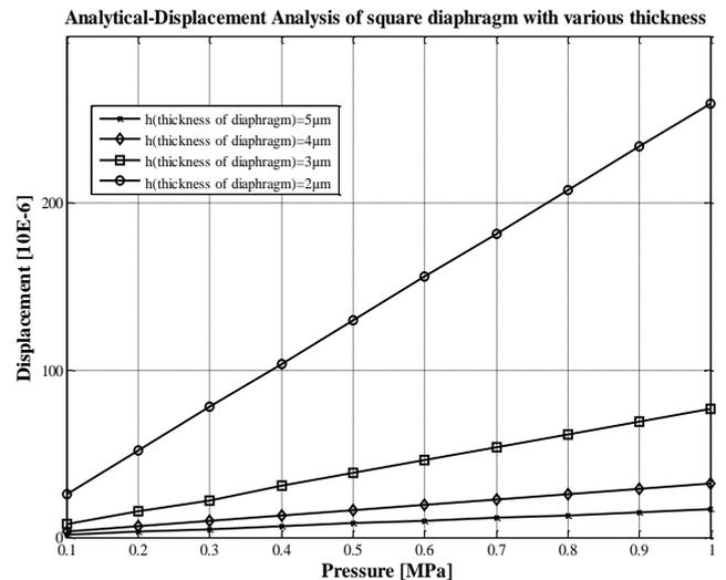
Fig.17. Analytical - Displacement analysis of various thickness of Square diaphragm
