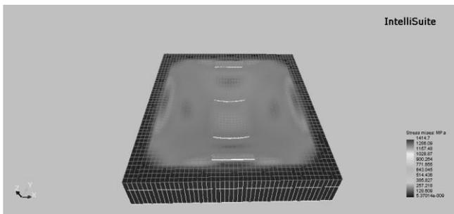
Fig.12. Mises Stress analysis of the Piezoresistive Pressure Sensor Model 3 with Pressure of 1MPa
