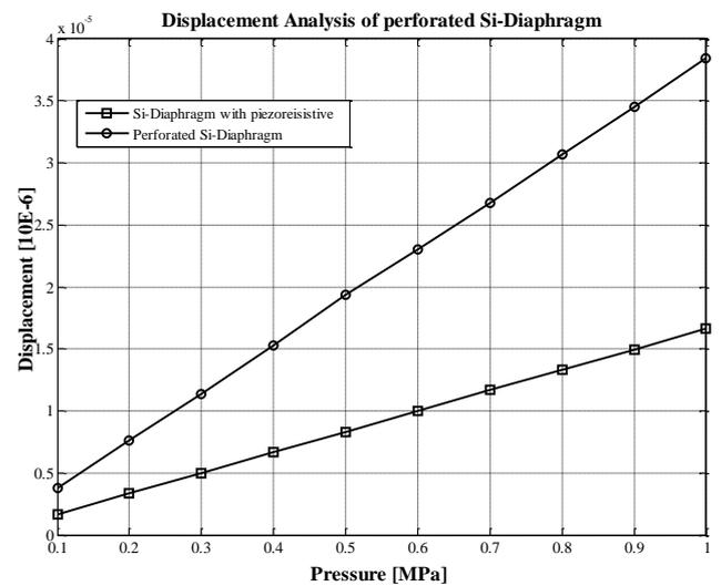
Fig.22. Displacement analysis of Perforated and Piezoresistive Si-Diaphragm
