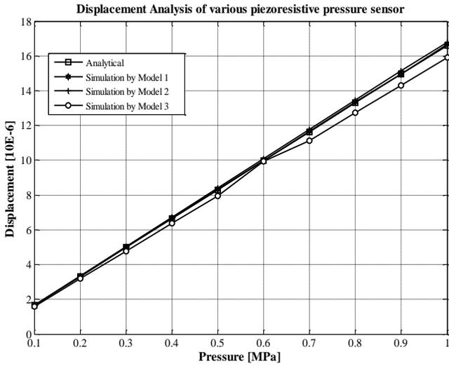
Fig.13. Displacement analysis of various piezoresistive pressure sensors with thickness at 5µm
