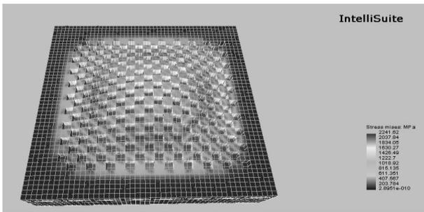
Fig.19. Simulation of perforated Si-diaphragm deformation on the Z axis with maximum pressure of 0.3MPa
