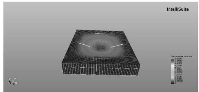
Fig.7. Simulation of Piezoresistive Pressure Sensor Model 1 deformation on the Z axis with maximum pressure of 0.5Mpa
