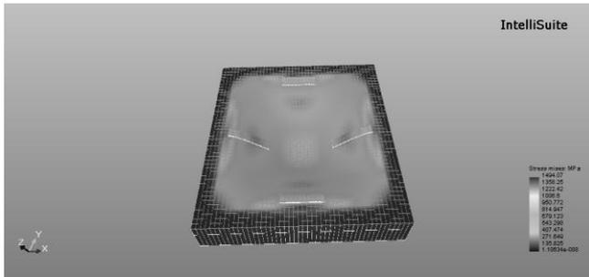
Fig.10. Mises Stress analysis of the Piezoresistive Pressure Sensor Model 1 with Pressure of 1MPa
