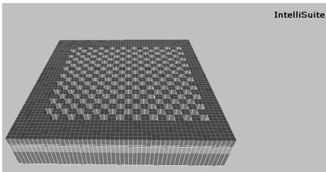
Fig.6. Proposed model of Perforated Si-Diaphragm Pressure sensor using 3D Builder
