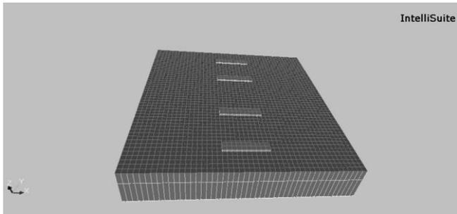
Fig.5. Si-Diaphragm with Piezoresistive Pressure sensor Model 3 Using 3D Builder
