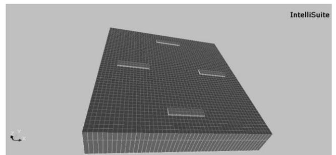
Fig.3. Si-Diaphragm with Piezoresistive Pressure sensor Model 1 Using 3D Builder
