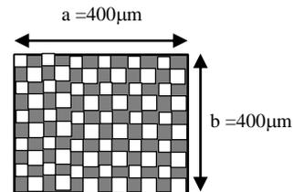
Fig.2. Schematic representation of proposed Perforated Si-diaphragm
