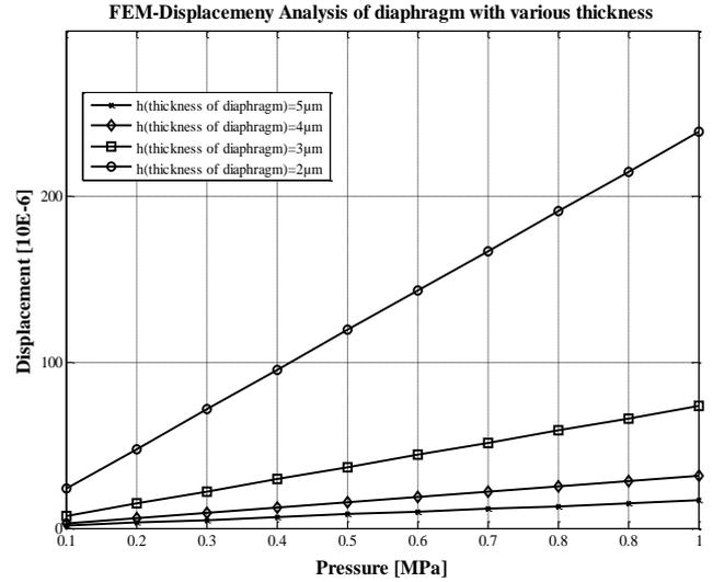
Fig.16. Finite Element Method (FEM)-Displacement analysis of various thickness of Square diaphragm
