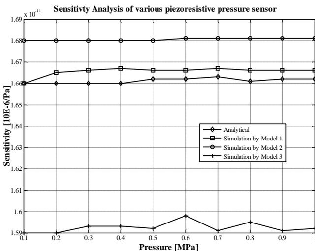
Fig.15. Sensitivity analysis of various piezoresistive pressure sensors with thickness at 5µm
