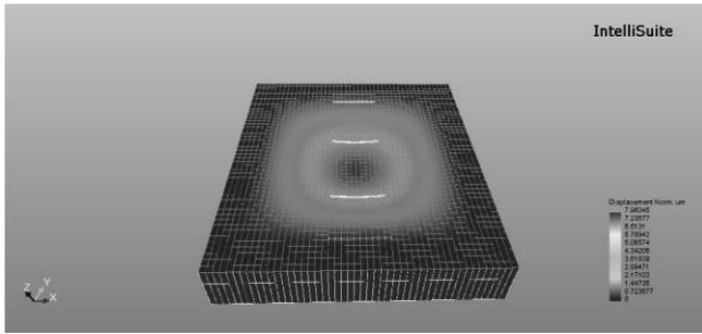
Fig.9. Simulation of Piezoresistive Pressure Sensor Model3 deformation on the Z axis with maximum pressure of 0.5Mpa
