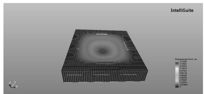
Fig.8. Simulation of Piezoresistive Pressure Sensor Model2 deformation on the Z axis with maximum pressure of 0.6MPa
