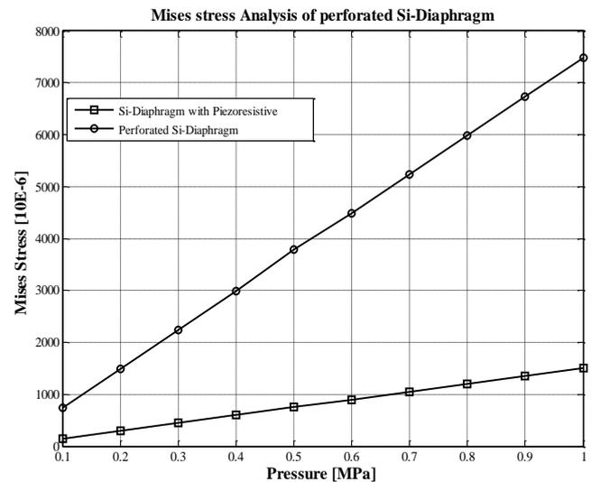
Fig.23. Mises Stress analysis of Perforated and Piezoresistive Si-Diaphragm
