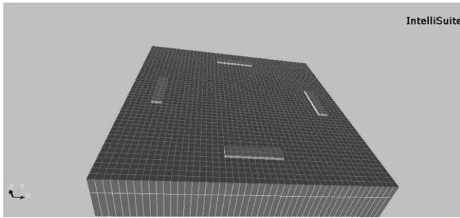
Fig.4. Si-Diaphragm with Piezoresistive Pressure sensor Model 2 Using 3D Builder
