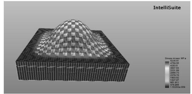
Fig.21. Mises Stress analysis of the perforated Si-diaphragm with Pressure of 0.7Mpa
