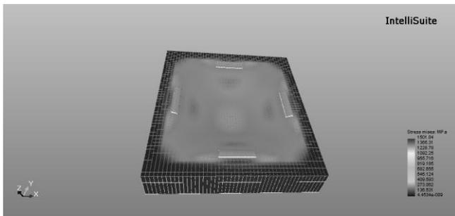
Fig.11. Mises Stress analysis of the Piezoresistive Pressure Sensor Model 2 with Pressure of 1MPa
