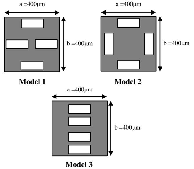
Fig.1. Schematic representation of various Models in Piezoresistive Pressure Sensor
