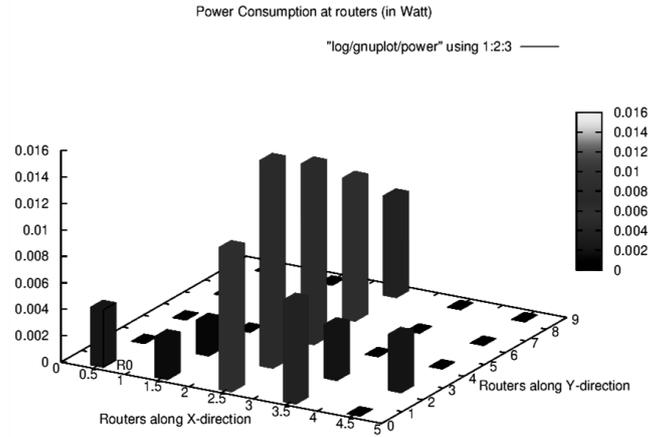
Fig.4. Power Consumption graph for PROM routing
