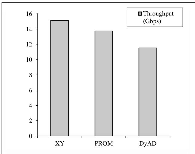
Fig.6. Throughput Analysis graph for routing techniques
