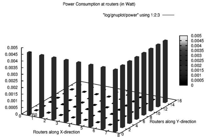
Fig.5. Power Consumption graph for DyAD routing
