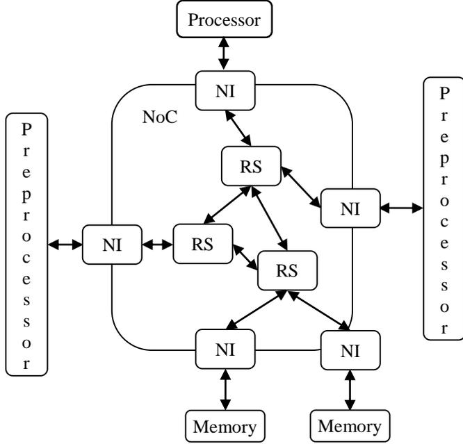
Fig.1. Basic Components of NoC Router
