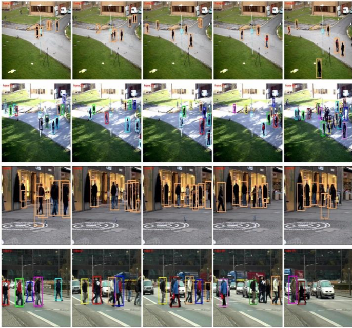
Fig.4. The tracking results of GEM-OT method: The rows 1,2,3,4 are the tracking video sequence of PETS2009 S2L2, PETS2009 S1L1-1, TUD-Stadtmitte and road crossing respectively
