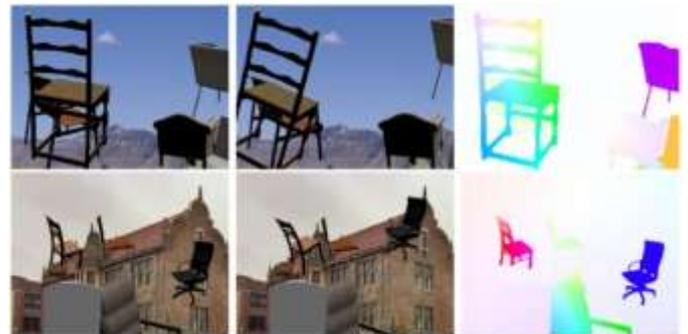
Fig.4. Synthetically generated data for training Optical Flow Models – Flying Chairs dataset
