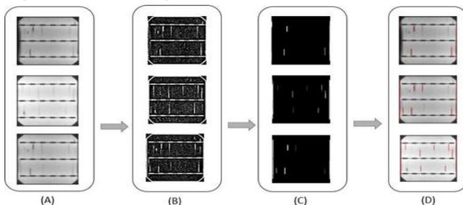
Fig.7. Shunt faults detection: (a) Solar cell images with shunt faults. (b) Edge detected images. (c) Vertical lines in the images indicating crack faults. (d) Shunt faults highlighted images.
