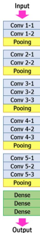
Fig.2. VGG16 CNN Architecture
