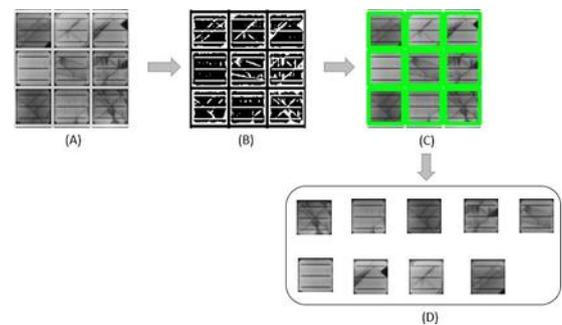
Fig.4. Solar cell segmentation: (a) Grayscale image with 9 cells. (b) Adaptive Gaussian thresholding applied on image. (c) Contour drawn image. (d) Segmented solar cells.
