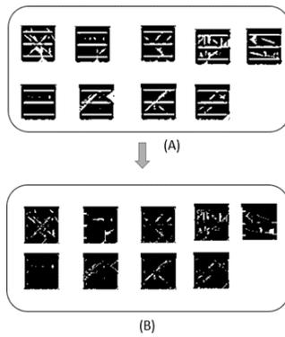
Fig.5. Crack faults detection: (a) Edge detected images (b) Horizontal line removed images showing crack faults.
