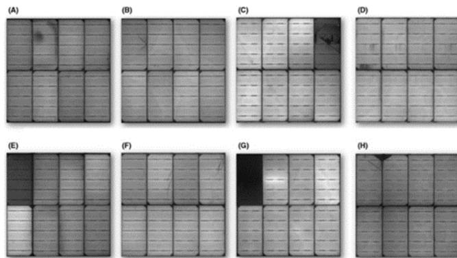
Fig.1. Types of defects in photovoltaic cells (a) Black area (b) Cracks (c) Break (d) Finger failure (e) Low cell (f) Scratches (g) Black cell (h) Broken corner. (i) Shunt faults.
