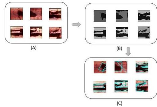
Fig.8. Black core and broken gate fault detection: (a) Solar cell images with black core/broken gate faults. (b) K-Means clustered images. (c) Black core/broken gate faults highlighted images.
