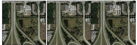
Fig.2. (a) Input Image of emerging suburban area (b) Result of bilateral Filtering (c) Histogram Equalization Processed Image
