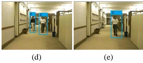
Fig.2. Multi object tracking results for 'hall monitor' video sequence using the proposed method for (a) frame 50, (b) frame 100, (c) frame 150, (d) frame 200, and (e) frame 250
