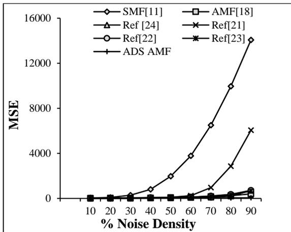
Fig.2. Mean Square Error (MSE) results comparison of the proposed and other filters
