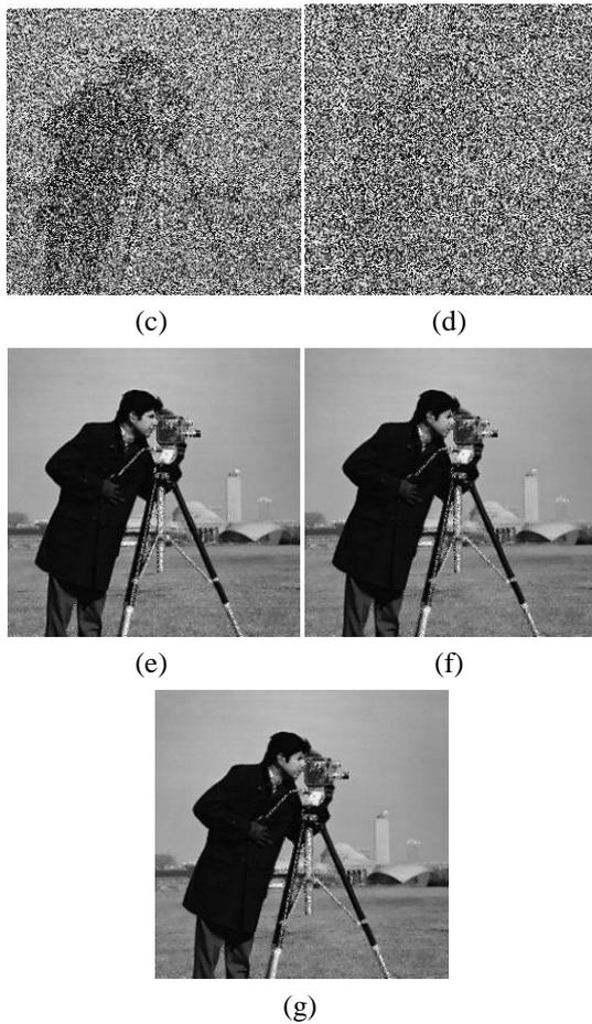
Fig.4. De-noising results of the proposed ADS-AMF (a) Original Cameraman image, (b-d) Noised at 70%, 80% and 90% density of salt and pepper impulse noise, (e-g) De-noised with the proposed ADS-AMF
