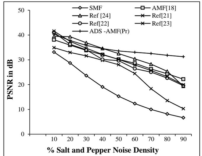
Fig.1. Peak Signal to Noise Ratio (PSNR) results comparison of the proposed and other filters
