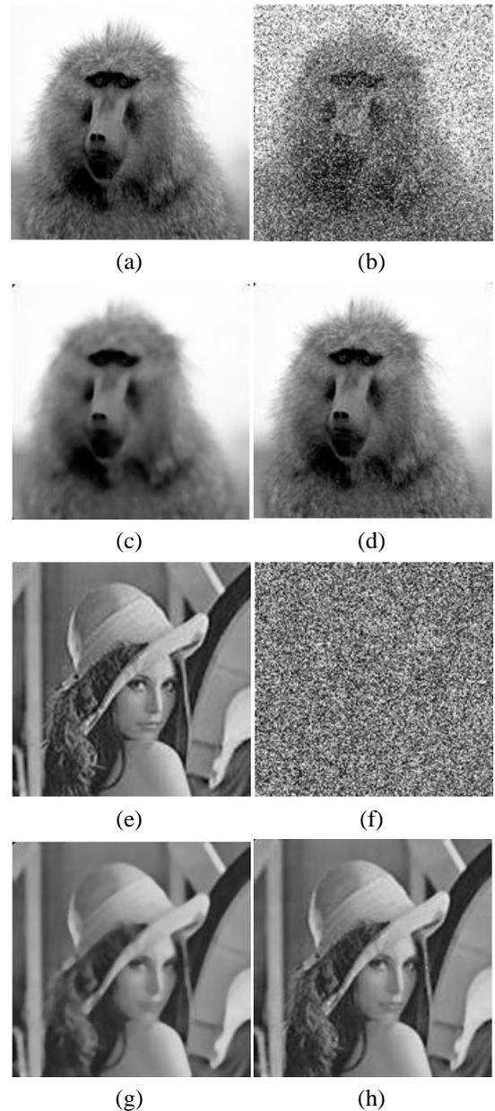
Fig.3. De-noising results of SMF and proposed ADS-AMF at 40% and 90% noise density for colour images, (a, e) Original Baboon and Lena images, (b, f) Noised at 40% and 70 %, (c, g) De-noised with SMF (d, h), De-noised with the proposed ADS-AMF
