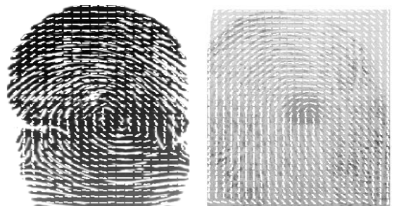
Fig.9. Reconstructed orientation of wet and dry images
