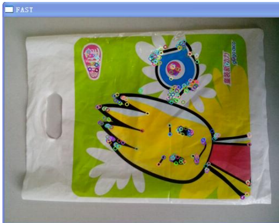
(a). Keypoints extracted by proposed method
