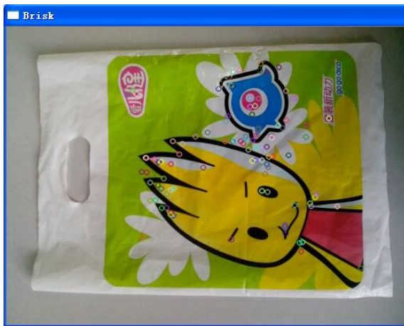
(b). Keypoints extracted by Brisk
