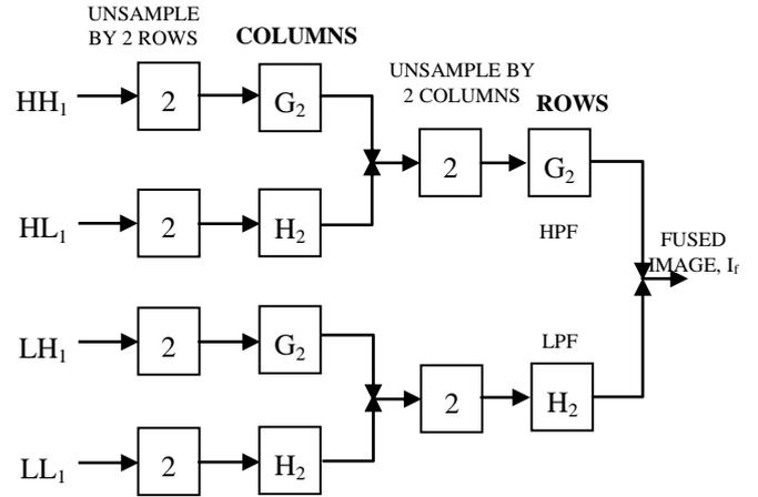
Fig.2. The DWT reconstruction part
