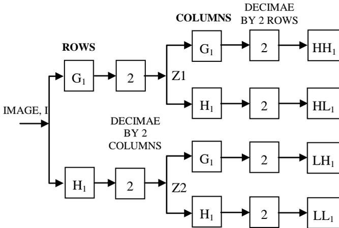
Fig.1. The DWT analysis part
