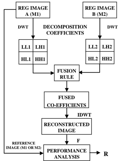
Fig.4. The proposed method block diagram
