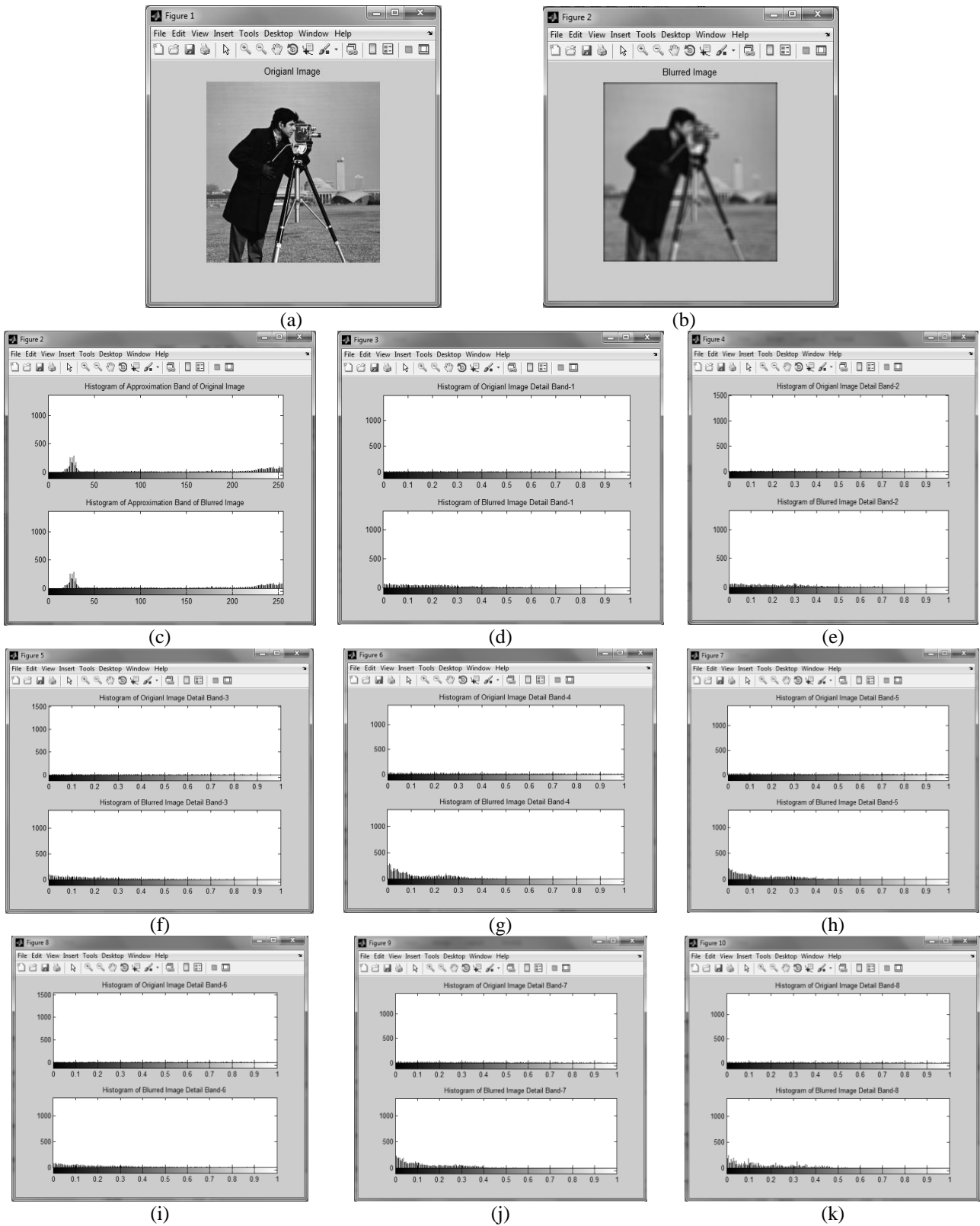
Fig.4. Histogram comparison of low and high frequency channel outputs of DDWT of sharp and blurred image (a). Sharper Image, (b). Blurred Image, (c). Histogram of Low frequency channel of Sharper (Upper Plot) and Blurred Image (Lower Plot) and (d) – (k). Histogram of 8-high frequency channels of Sharper (Upper Plot) and Blurred Image (Lower Plot)
