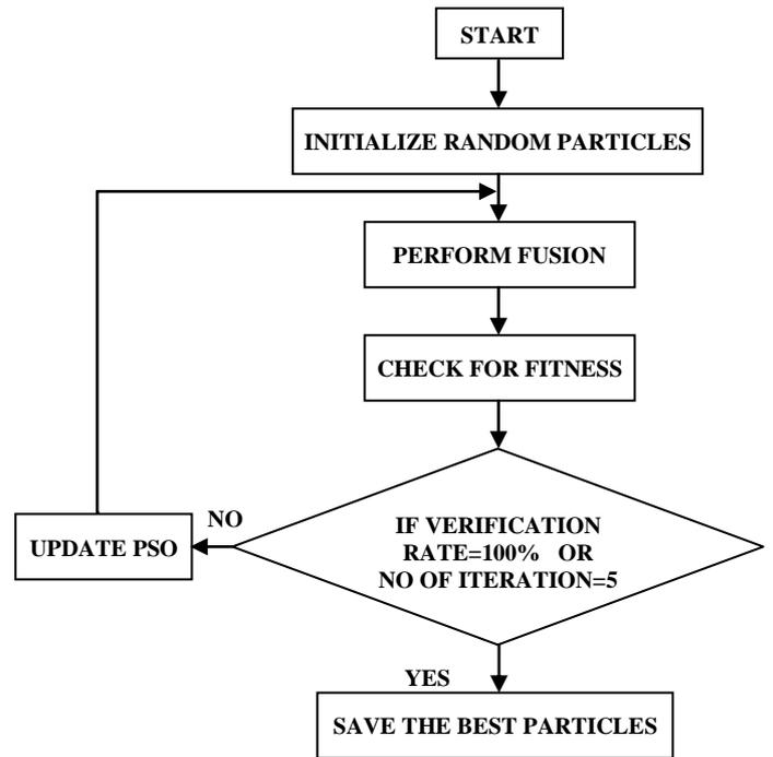
Fig.5. Flow diagram of PSO
