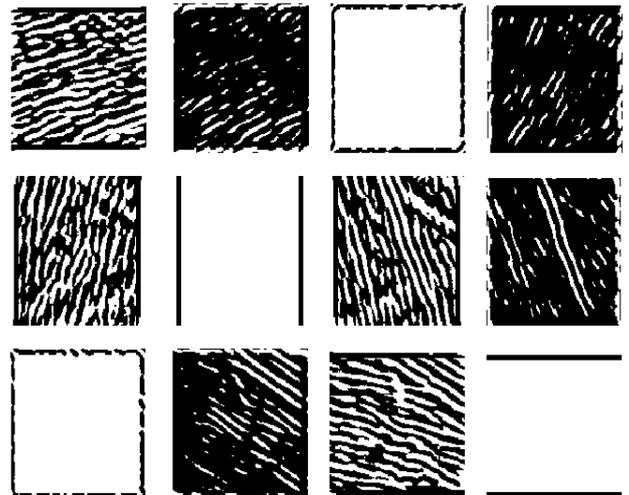
Fig.3. Filtered images using Gabor filter with twelve orientations
