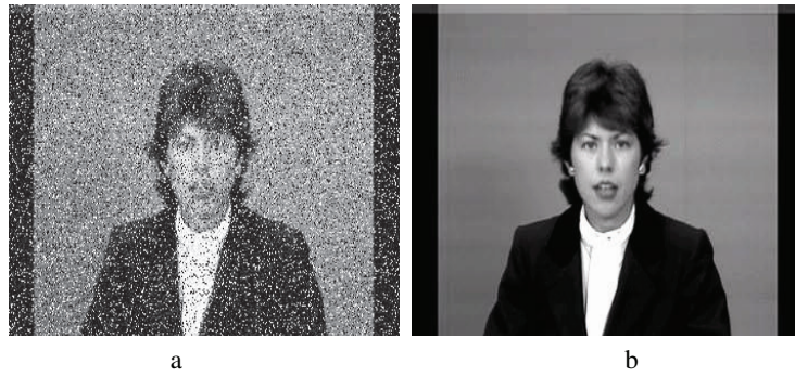
Fig.8. (a) Frame 28 from Claire video sequence corrupted by 30% impulse noise and Gaussian noise of \sigma = 20 (b) Restored image
