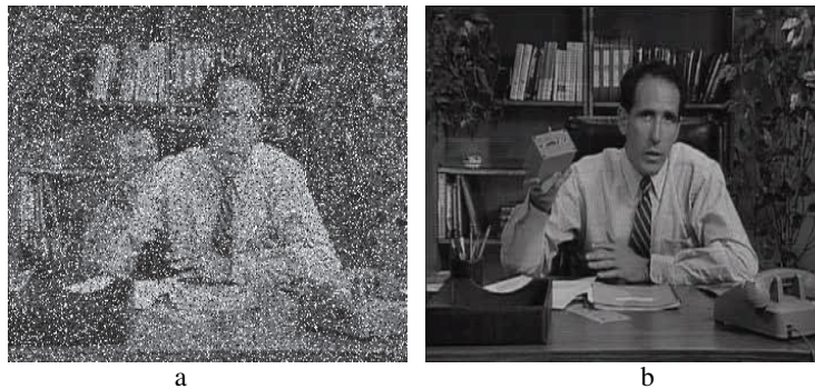
Fig.9. (a) Frame 16 from Salesman video sequence corrupted by 30% impulse noise and Gaussian noise of \sigma = 20 (b) Restored image
