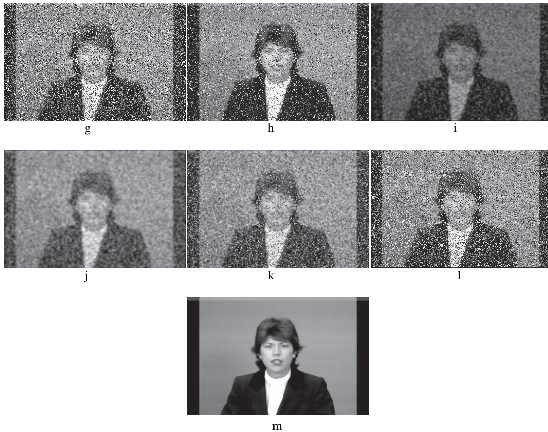
Fig.4. Results of different filters for frame 16 of Claire video sequence. (a) Original Sequence. (b) Image sequence corrupted by 30% salt & pepper noise and \sigma=20 . (c) Output of SMF. (d) Output of PSMF (e) Output of AMF. (f) Output of RAMF. (g) Output of DBA. (h) Output of REMF. (i) Output of ATMF. (j) Output of Mean filter (k) Output of Wiener filter. (l) Output of Bilateral. (m) Output of PA
