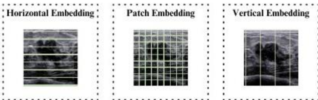
Fig.2. Patch and Strip Embeddings: Three embedding types used in AnatoFormer. Horizontal embedding aligns with anatomical layers, patch embedding extracts local features, and vertical embedding captures inter-layer dependencies.
